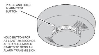
STEP 9 Complete receiver programming. Refer to the instructions supplied with the supervised receiver to program the TSD-90A as a 24-hour fire alarm. Repeat the previous step to verify that the TSD-90A triggers the correct zone on the receiver and that the correct report is sent to the central station (if the system is monitored).
