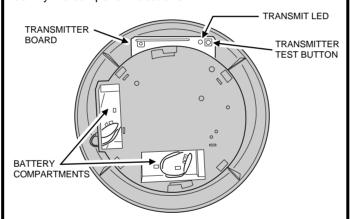
**STEP 3** *Install batteries.* Connect the two 9-volt batteries and place them into battery holding cups.
