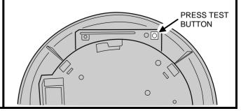
STEP 7 Attach TSD-90A to mounting plate. Match up alignment tabs on alarm and plate. Turn alarm clockwise until it locks in place (tamper switch will click as alarm locks onto plate).
